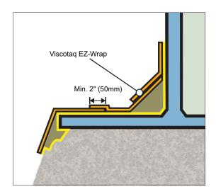
5.3.5 The Viscotaq EZ Wrap shall be gently smoothed by hand and steel roller to ensure there are no wrinkles, folds, or entrapped air. If required you may use a heat gun and pressure to make sure the sealing compound is fully impregnated in the polyester backing of the Viscotaq EZ Wrap.
