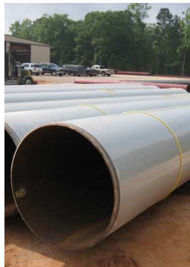
Pipe coated with 30 mils of Protal 7900HT.
